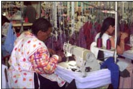
Production in SA - with a rail system to eliminate/reduce bundling and handling.
